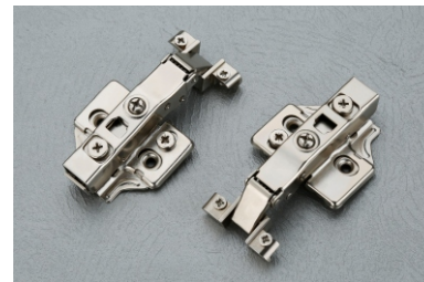
KAH - 04 Clip On Profile Auto Close Crank : 0°, 8°, 16° Finish : Zinc
